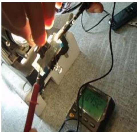
Fig 1. Test of the voltage supplied by the solar cell
